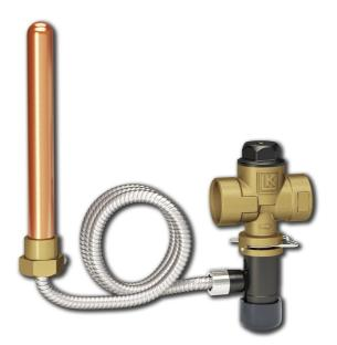
LK 519 ThermoSafe is a thermal safety valve for solid fuel boilers with built-in water heaters or cooling coils. The safety valve prevents the temperature of the boiler water from rising above the boiling point. When temperature levels are too high the valve opens to let cold water flow through water heater or cooling coil, thus reducing the temperature of the boiler. LK 519 ThermoSafe has two, separately functioning, temperature sensors for added safety.
