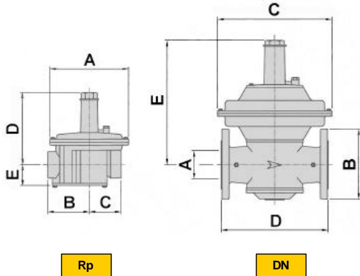
Dimensioni in mm - Dimension in mm
