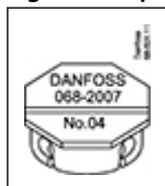
Figure 7: Capillary tube label for T2 and TE2
