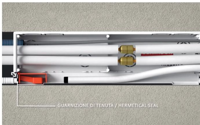
**EN** Once discharge has finished, the FREESTOP system lowers automatically closing hermetically the drain duct thanks to the O-ring gasket supplied, differently to what happens with rough-in box with siphon, where condensate evaporation caused by a long non-use of the air conditioner (eg. from approx. September to May) may favor the passage of bad smells as shown in the example.
